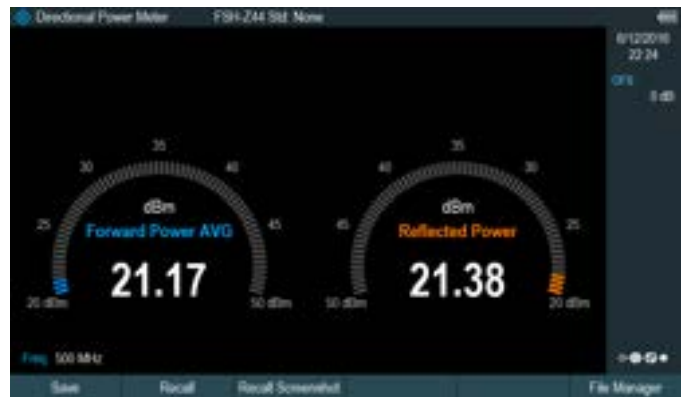
Forward and reflected power measurement with directional power sensor (R&S®FSH-Z44).
