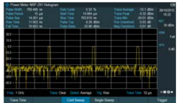
Pulse analysis with R&S®ZNH-K29 and R&S®NRP-Z81 wideband power sensors.
