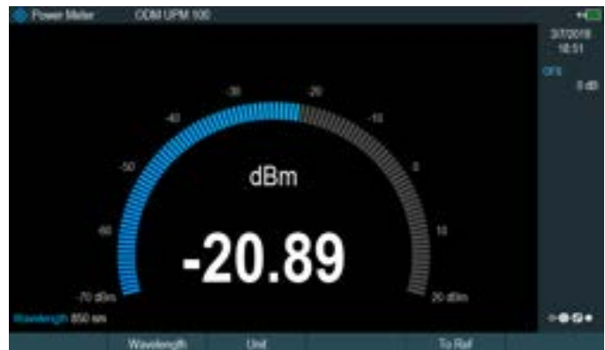
Optical power measurement with optical power sensor.
