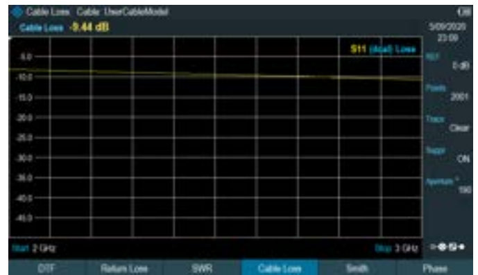
One-port cable loss measurement.
