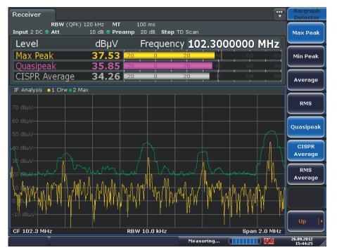
Upper part of screen: Combined numeric and bargraph level display for the current receive frequency with up to four different weighting
